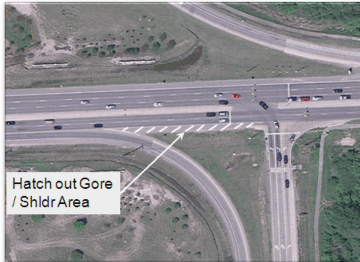
Figure 4.13 – Potential Gore/Shoulder Hatching at the EB M-153 to NB I-275 Entrance Ramp
