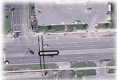
Figure 4.8 – Potential Pedestrian Refuge Island with Signalized Cross-Walk
