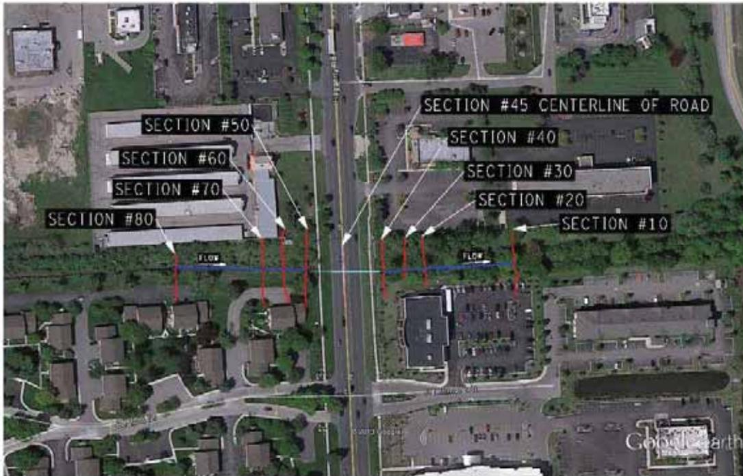
Figure 2 - Aerial Photo Showing Approximate Cross-Section Locations
